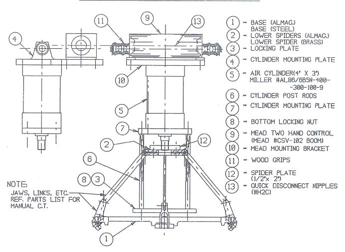
HEIGHT OF HAND/AIR SEMI-AUTOMATIC BOOM TYPE CLOSING TOOL FROM BOTTOM OF JAW TO THE TOP OF THE TWO HAND CONTROL UNIT ..... 19-1/2"
